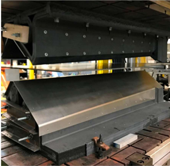
Figure 6.0 AM mold set in press. Sheet Metal cladding is clearly visible on the plug mold.
