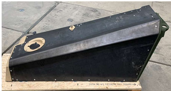
Figure 1.0 Carbon/PPS composite vehicle component fastened to vehicle end cap and pillar components, ready for assembly to vehicle.
