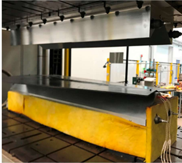
Figure 4.0 Fabricated metallic mold set. Plug mold is mounted to the press' bottom platen. Cavity mold is mounted to the press' upper platen.
