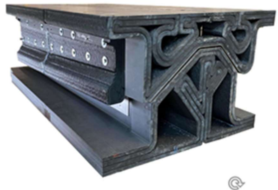
Figure 6.0. Complete AM ABS/Sheet metal Clad, Compression Mold Set.
