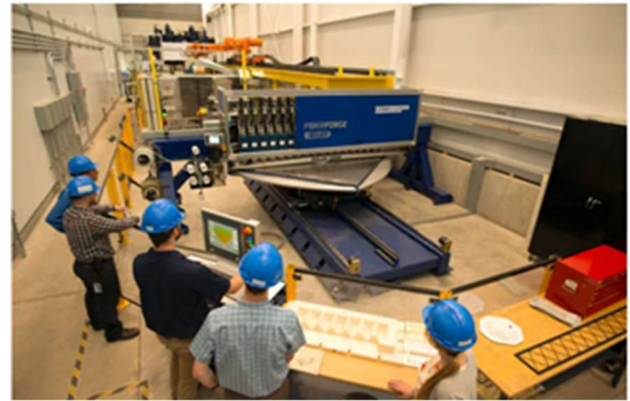
Figure 8.0 Dieffenbacher-FiberForge RELAY system located at the University of Maine
